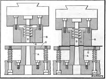
Fig. 4. Compound Die which Pierces and Blanks Simultaneously
